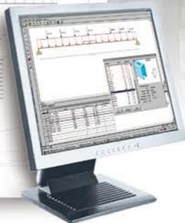
UNISTRUT analysis Software: A user friendly, two dimensional calculation program to analyze UNISTRUT channel sections utilized as beams and cantilevers. The program provides instantaneous results of geometries containing multiple spans with single or multiple static load conditions
